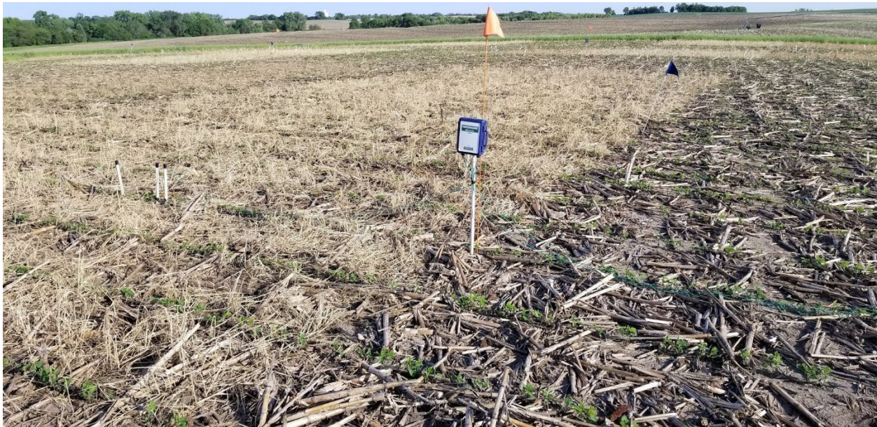
Image 1. Watermark soil water sensors installed at SMFD plot.
